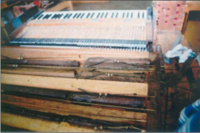
cells is that they have been installed in a vertical position, with the openings to the reed cells facing upward, instead of the usually horizontal configuration. This configuration offers better access to the reed for servicing. The Swell shades are two large wooden flaps that open sideways.
