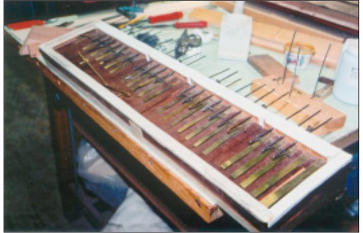
of a bourdon. Because of the amplitude of their travel, the tongues are prone to frequent breakage.
